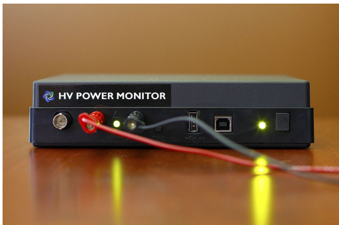
Fig. 2. High voltage power monitor from Msoon Solution [20]
